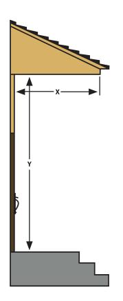
Adequate overhang is very critical to the life and performance of a wood stile and rail door.
