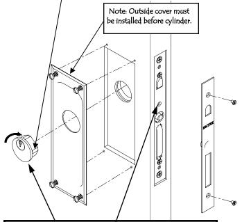
After threading both inside & outside cylinders into lock body, tighten locking screw counter clockwise to engage notches on both cylinders.
