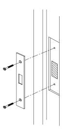
Drill two 1/8" pilot holes for wood screws provided).
